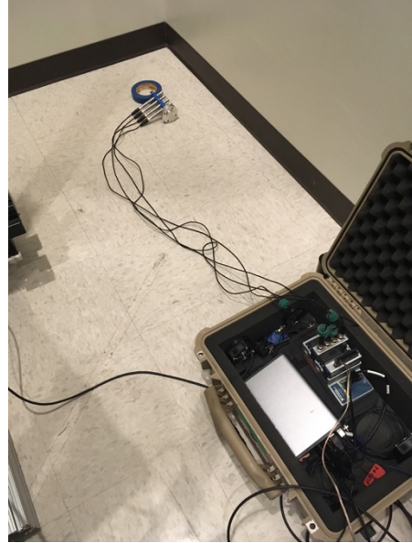
Figure 2.2.11 Reverberation chamber experiment layout. Two subwoofers were placed in the corner of the room facing against the wall. Microphones were located on the floor at the other corner of the room using the same array configuration used in the car.
